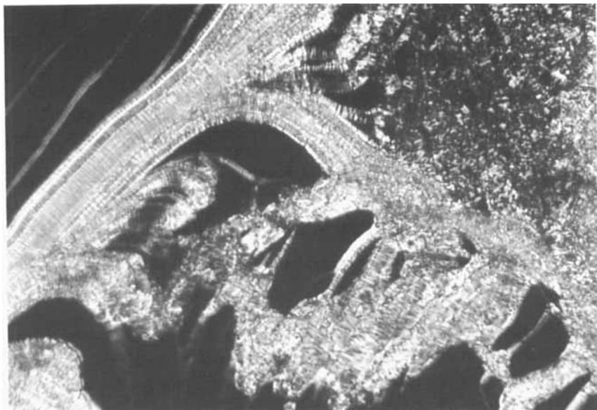
FIGURE 3 The characteristic oily streak pattern of the S_A phase of C16MO at 120°C formed on heating the crystal (at the rate of 10°C/min) (See Color Plate III at the back of this issue)
