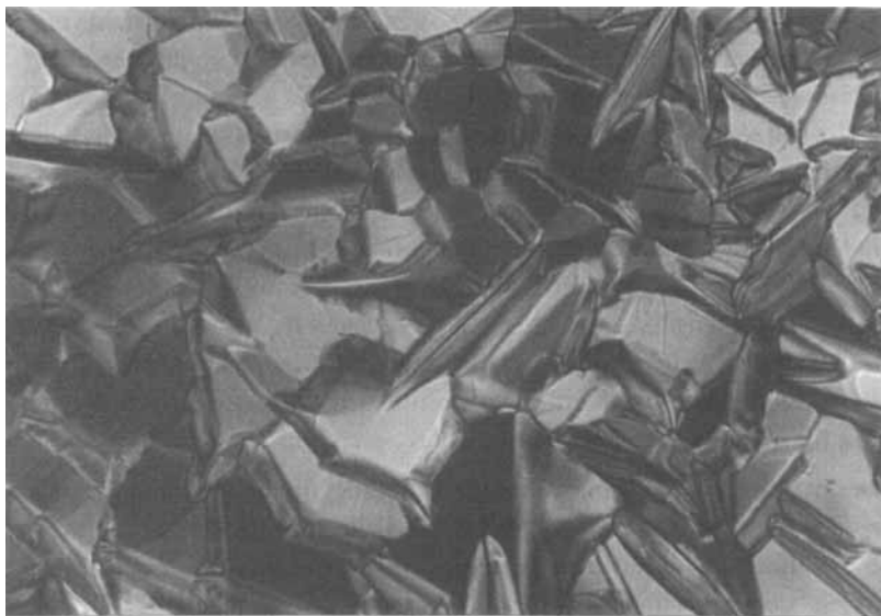
FIGURE 1 The characteristic mosaic and lancet texture of the S_B phase of C8M at 80°C (See Color Plate I at the back of this issue)
